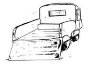
A ramp is used for loading this truck. A mover can pull a cart with a heavy object up the ramp. This is much easier than lifting heavy objects into the truck.
