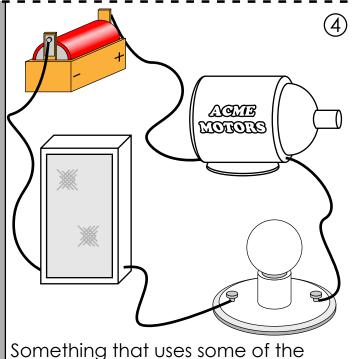
Something that uses some of the electricity in a circuit is called a resistor. Resistors could also be things
