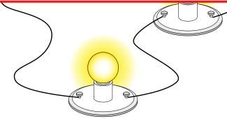
The picture above shows a circuit. Electricity flows from the negative side of a battery, through the wires, and lights the bulb. The electricity continues to travel around to the positive side of the battery.
