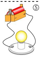
A circuit can be open or closed. When a circuit is closed, it is complete and there is no break in the path that the charges must follow. When a circuit is open, it is incomplete and charges can't flow through.
