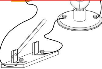
A switch is sometimes added to a circuit. The switch opens and closes a circuit to turn resistors on and off.
