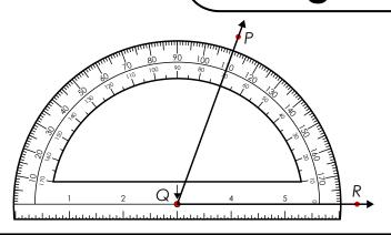
The protractor's arrow and pen hole is placed on the angle's vertex. The 0° line is placed over one side of the angle. Read the measure where the other leg of the angle intersects the protractor.
